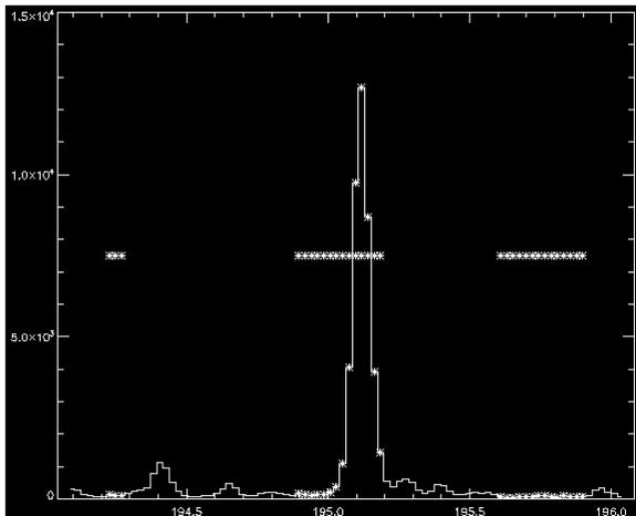
Now we need to tie the line parameters of the 195.18 line to those of 195.12. I assume that 195.12 is represented by Gaussian 0 (i.e., the first line clicked in `eis_fit_template`):
